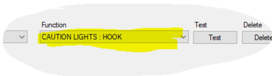
The "Function" column corresponds to the function of the lightBit in the Falcon BMS simulator. I invite you for testing to use a simple function like the "Hook" or the seat lock that immediately lights the PFL.
